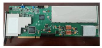
Fig. 2. Ultrasonic flaw detection card.
