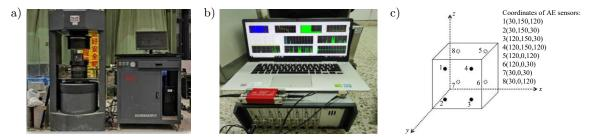
Fig. 2. Test apparatus: a) HCT306B press; b) AMSY-6 acoustic emission instrument; c) acoustics emission sensor arrangement (applied load acts parallel to the z-axis on the plane above the specimen).
