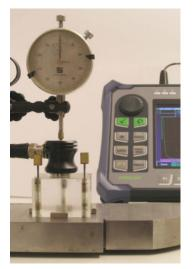
Fig. 4. Photograph of the experimental setup to determine CL, introduced by water coupling layer existing between a PMMA delay line and a steel block.
