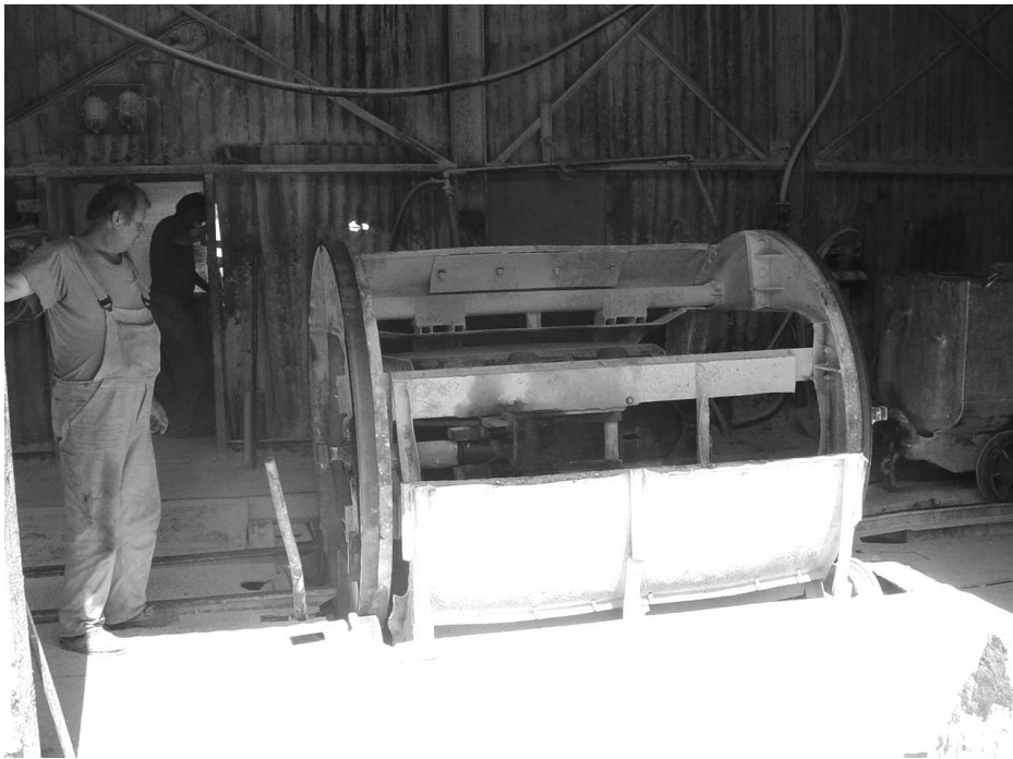
Fig. 8. Dumping conveyer feeding the crusher with stones from wagons.
