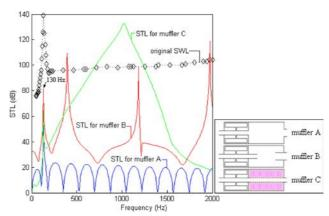
Fig. 7. Comparison of the original SWL (hybridized with a pure tone - 130 Hz) with respect to the STL at various mufflers [muffler A; a one-chamber HR element and a one-chamber simple expansion element; muffler B; a one-chamber HR element and a one-chamber tube-extended element; muffler C; a one-chamber HR element and a one-chamber dissipative element].
