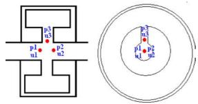
Fig. 9. A one-chamber Helmholtz resonator (HR) muffler.
