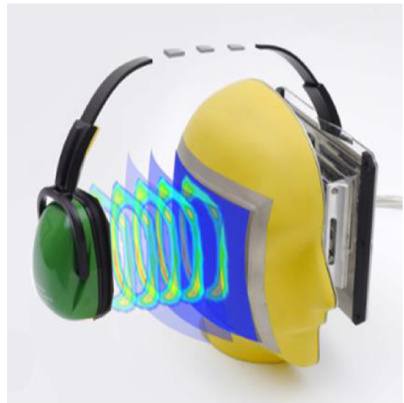
Fig. 3. Conformable tactile sensor elements (manufactured by PPS), one on each side (see Fig. 2). Permanent fixed sensors. Each side has 1024 sensors over an area of 3.8 \times 3.8 \text{ mm} .
