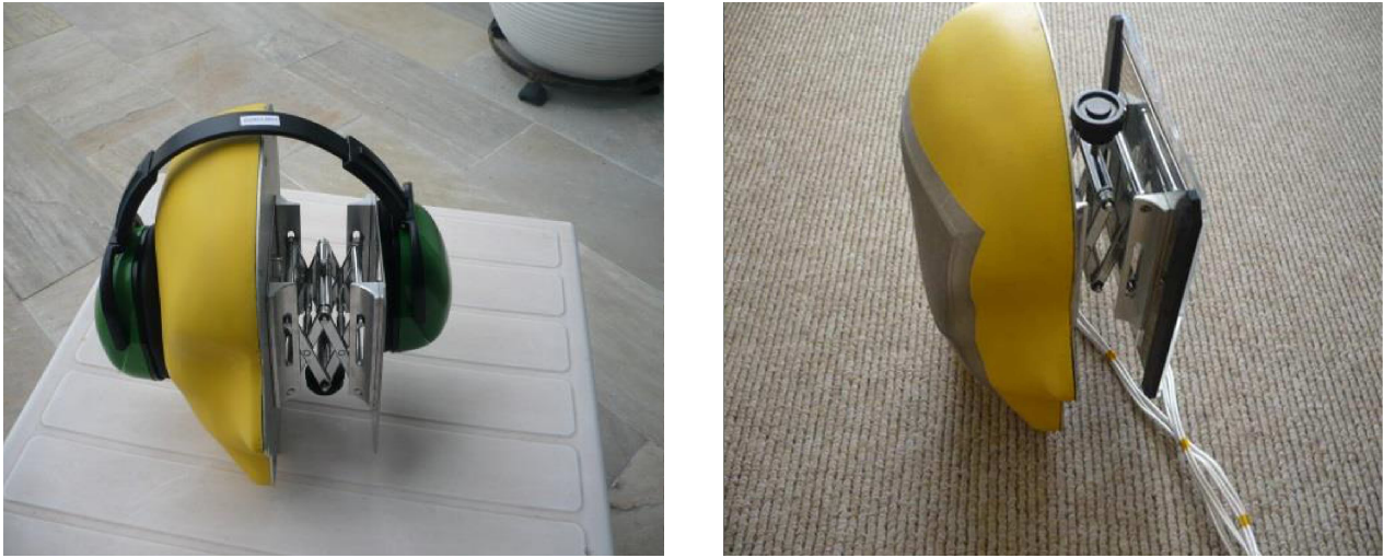
Fig. 4. Variable width measurement systems with flat surface on one side and half dummy human head on the other side.
