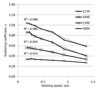
Fig. 4. Sound scattering coefficient determined using sine sweep signal as a function of turntable rotational speed for selected frequencies ( $\mathbb{R}^2$  is a coefficient of determination).
