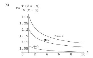
Fig. 1. a) Excess density of acoustic pulse  $\rho_a(x,t=1)$  corresponding to the following quantities of C: 1.5,2,5,-5,-2,-1.5, from the lower curve to the upper one. b) A ratio  $r(\eta,t)=\Phi(C=-\eta,t)/\Phi(C=\eta,t)$  for values of  $\eta$  as follows: 5 (lowest curve), 2 (middle curve) and 1.5 (upper curve).  $\Phi(C,t)=q_e/\int\limits_0^\infty \rho_a^2(x,t=1)\mathrm{d}x \text{ denotes the efficiency of heating.}$
