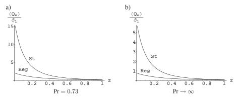
Fig. 3. Heating produced by stochastic (upper curve) and regular (lower curve) periodic sound  $Q_e$ , divided by viscosity  $\delta_1$ , as a function of  $z=\frac{\gamma+1}{2}\sigma x$ ; x denotes dimensionless distance from a transducer. Calculations are in accordance to the formula (11) with the acoustic velocity (18).
