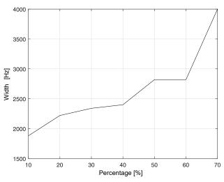
Fig. 5. Width of insertion loss peak as a function of filling fraction.
