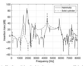
Fig. 8. ILs for solid cylindrical scatterers versus Helmholtz resonant scatterers.
