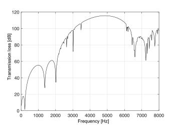
Fig. 3. STL of DPS with  $7 \times 2$  cylindrical scatterers arranged on square lattice.
