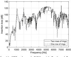
Fig. 10. STLs through DPSs with  $7\times 2$  and  $7\times 3$  hybrid SCs.
