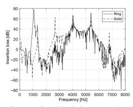
Fig. 7. IL spectra for solid cylinder arrays and ring-type scatterers.
