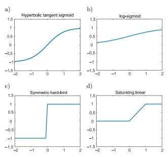
Fig. 1. Four types of neural network activation functions: a) hyperbolic tangent sigmoid, b) log-sigmoid, c) symmetric hard-limit, and d) saturating linear transfer functions.
