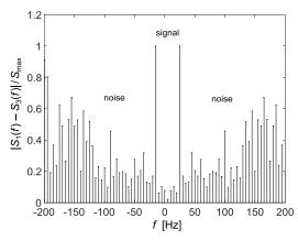
Fig. 19. Spectra difference of signal with noise received by hydrophones (parameters as in Fig. 18).
