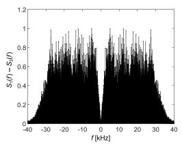
Fig. 15. Difference of noise spectra from Fig. 14.
