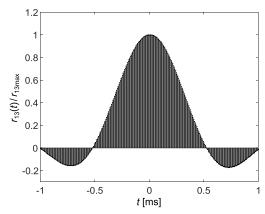
Fig. 12. Noise correlation function with spectrum width  $B=1~\mathrm{kHz}.$
