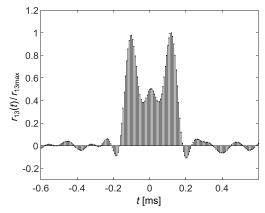
Fig. 13. Noise correlation function with spectrum width  $B=10~\mathrm{kHz}.$
