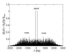
Fig. 23. Spectra difference of signal with noise received by hydrophones (parameters as in Fig. 22).
