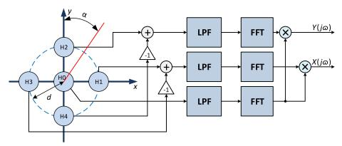
Fig. 1. Functional diagram of a DIFAR system.
