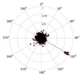
Fig. 18. Example bearing at frequency  $f_0 = 20 \text{ Hz}$  (2d = 0.4 m,  $f_s = 150 \text{ kHz}$ , B = 2 kHz, T = 0.2 s, SNR = 0 dB, N = 10000,  $\alpha = 120^{\circ}$ ).
