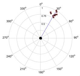
Fig. 22. Example bearing for non-correlated noise (2d = 0.2 m,  $f_s$  = 150 kHz, B = 2 kHz, T = 0.1 s, SNR = 15 dB, N = 10000,  $\alpha$  = 30°,  $r_{p13}$  = 0.023.
