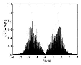
Fig. 7. The spectra difference of noise received by hydrophones 1 and 3 (parameters as in Fig. 5).
