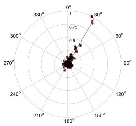
Fig. 21. Rectangular wave bearing ( $f_0 = 100 \text{ Hz}$ , 2d = 0.2 m,  $f_s = 150 \text{ kHz}$ , T = 0.2 s, SNR = 5 dB, N = 10000,  $\alpha = 30^{\circ}$ ).
