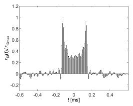
Fig. 14. Noise correlation function with spectrum width  $B=30~\mathrm{kHz}.$
