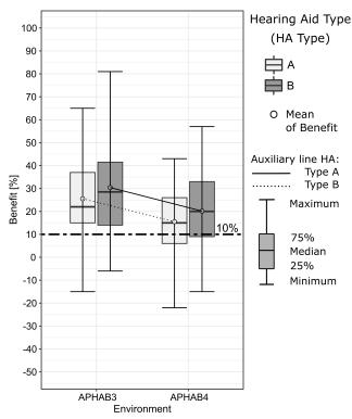
Fig. 1. Benefits obtained during short-term use of hearing aids with different technology levels, presented in the form of global indicators for three and four environments respectively (HA refers to hearing aid).
