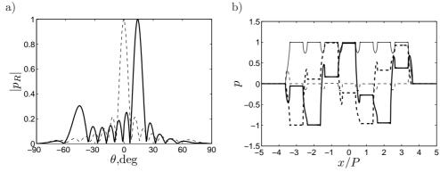
Fig. 2. a) Far-field radiation pattern for an 8 element baffle array; steering angle  $\beta = 15^{\circ}$  (a solid line) and  $\beta = 0^{\circ}$  (a dashed line);  $P = \lambda$ ,  $w = 0.75\lambda$ ; b) spatial distribution of p(x) on the baffle plane; steering angle  $\beta = 15^{\circ}$  (thick lines) and  $\beta = 0^{\circ}$  (a thin line); solid lines  $-\operatorname{Re}(p)$ , dashed lines  $-\operatorname{Im}(p)$ .
