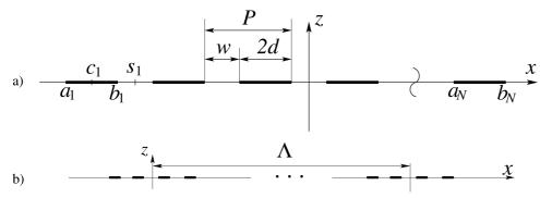
Fig. 1. a) A system of N rigid baffles (strips) on the boundary of acoustic media spanning for z > 0; b) multi-periodic structure with certain large period  $\Lambda$  comprised by the replicas of the finite baffle system (a).
