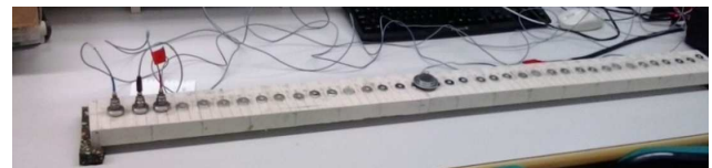
Fig. 4. Detailed view of a section of the experimental setup. Top: location of the source (actuator) 2 cm away from the left edge of the beam. Bottom: three accelerometers near the left edge of the beam and an actuator in the centre.
