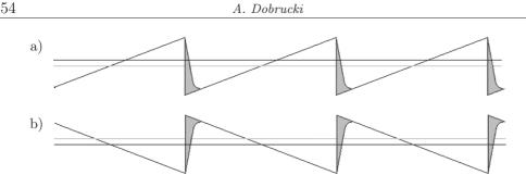
Fig. 15. Sawtooth signals used in the IS method, a) increasing slope slow, decreasing – fast, b) decreasing slope slow, increasing – fast.
