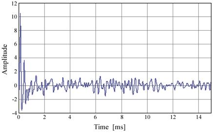
Fig. 3. Wiener kernel of the order 1 of an electrodynamic loudspeaker (Dobrucki, Pruchnicki, 2001).
