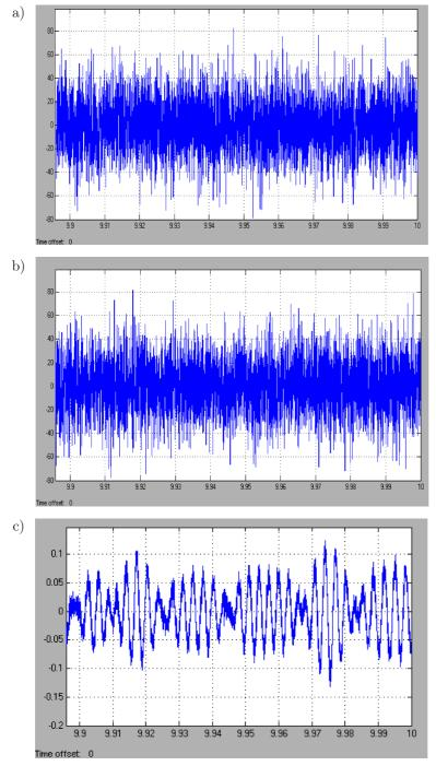
Fig. 9. Signals in various points of setup for measurement of nonlinear distortion using Wolf's method, a) signal from noise generator, b) signal after band-stop filter, c) signal after band-pass filter. X-axis: time in seconds, Y-axis: amplitude in arbitrary units.
