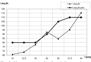
Fig. 5. Measurements results of equivalent sound pressure levels at workstation of ultrasonic washer Sonic 5  $(L_{\rm feq,8h,adm.} = MAL)$  (SMAGOWSKA, 2015; cit. with the author's kind permission).
