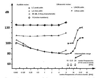
Fig. 6. A comparison of the curves for evaluation of admissible values for audible noise and for ultrasonic noise at work places  $L_{\text{fe.8h.adm}}$  and  $L_{\text{fmax.adm}}$ , respectively (cit. ŚLIWIŃSKI, 2013) with several alterations.
