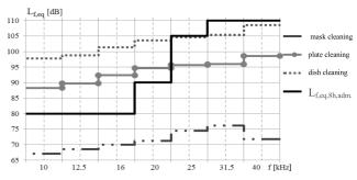
Fig. 4. Measurements results of equivalent sound pressure levels at workstations with cleaning units using compressed air ( $L_{\rm feq,8h,adm} = MAL$ ) (SMAGOWSKA, 2013; cit. with the author's kind permission).
