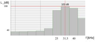
Fig. 3. Ultrasonic noise spectrum of the medium (M) sound pressure level (SMAGOWSKA, MIKULSKI, 2012; cit. with the authors' kind permission).
