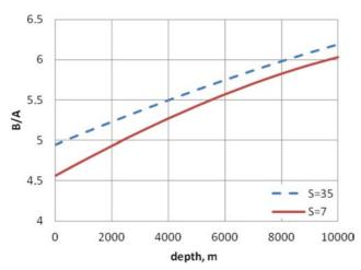
Fig. 2. Changes in nonlinearity parameter B/A in sea water of temperature 5°C as a function of depth for salinity S=7 PSU and S=35 PSU.
