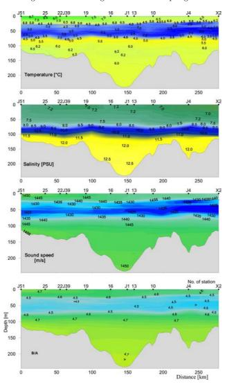
Fig. 6. Vertical distribution of temperature, salinity, sound speed and B/A in May at the Gotland Deep along transect shown in Fig. 5.
