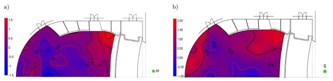
Fig. 14. The effect of mounting the diffusers on the sound strength G in octave bands: (a) 0.5–1 kHz and (b) 4 kHz.
