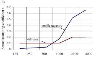
Fig. 11. Acoustic parameters of the textile tapestry and the diffuser of Fig. 9 used in computer simulation (octave resolution, frequency range 125–4000 Hz): a) sound absorption coefficient  $\alpha$ , b) sound scattering coefficient s (Kamisiński et al., 2012b).
