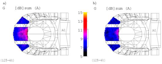
Fig. 12. The forecasted distribution of G values in the underbalcony area for the rear wall covered with: a) textile tapestry, b) sound diffuser.
