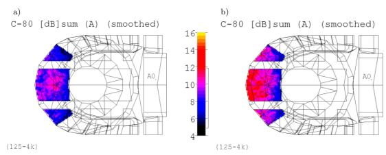
Fig. 13. The forecasted distribution of  $C_{80}$  values in the underbalcony area for the rear wall covered with: a) textile tapestry, b) sound diffuser.
