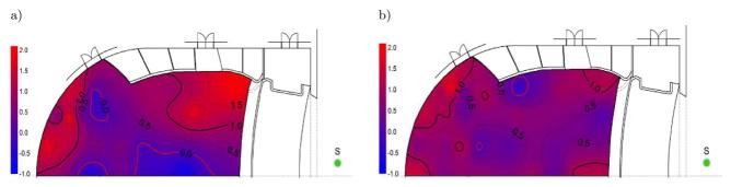
Fig. 15. The effect of mounting the diffusers on the sound strength G: a)  $G_{80 \text{ ms}, 4k}$  and b)  $G_{\text{Late}, 4k}$ .
