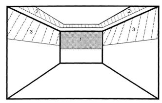
Fig. 3. The recommended sequence in which the soundabsorbing materials should be applied, in the order corresponding to increasing effect on the room acoustics: 1 – rear wall; 2 – ceiling portions bordering to walls, 3 – upper portions of side walls (Kulowski, 2011; Fasold, Winkler, 1976).
