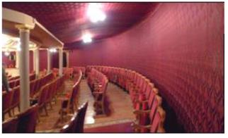
Fig. 8. The underbalcony space in the Lviv Opera House hall prior to installing the sound diffusing structures. The walls and ceiling were covered with a textile tapestry.
