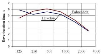
Fig. 21. Reverberation time of the courtyards after textural plaster renovation and face brick cleaning (July 2007).
