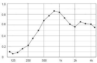
Fig. 24. The sound absorption frequency characteristic for the microperforated foil stretched at a distance of 10 cm from glass pane. Film parameters: thickness 0.18 mm; 500,000 Ø0.1 mm holes per m<sup>2</sup>; perforation rate 1%; sound absorptivity class D,  $\alpha_w = 0.55$  (NOCKE, 2014).
