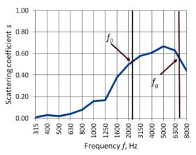
Fig. 10. The sound scattering coefficient s for the diffuser of Fig. 9 obtained from acoustics measurements (third-octave resolution, frequency range 314–8000 Hz).  $f_0$  and  $f_g$  are the lower and the higher sound diffusion limiting frequencies, respectively. It is assumed that sound diffusion occurs at frequencies above 0.5  $f_0$  (KAMISIŃSKI  $et\ al.$ , 2012b).
