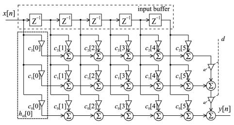
Fig. 7. Farrow structure of order q = 2 implementing VFD filter of length N = 6.
