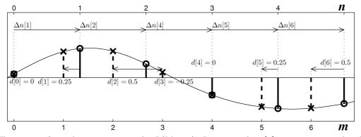
Fig. 2. Illustration of sample rate conversion by L/M = 5/4. Input samples  $x[n] - \circ$ , output samples  $y[m] - \times$ .
