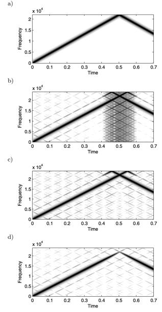
Fig. 6. Spectrograms illustrating resampling with constant resampling ratio 160/147 using VFD filters from Fig. 5 implemented with the Farrow structure of order q = 5: a) input chirp signal, b) signal resampled using minimax FD filters ( $f_{\rm a} = 0.4$ ), c) signal resampled using fullband ( $f_{\rm c} = 0.5$ ) FD filters designed using offset window, d) signal resampled using FD filters designed using offset window for  $f_{\rm c} = f_{\rm a}$ .
