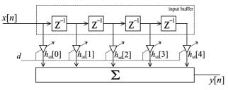
Fig. 3. General VFD filter structure applied to SRC.
