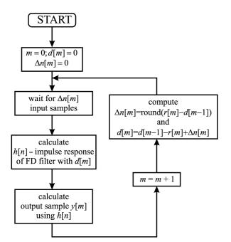
Fig. 4. Diagram of SRC algorithm based on VFD filter.
