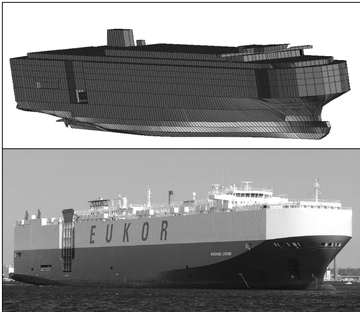
Fig. 1. RORO ship “MORNING CROWN” with Finite Element Model.
