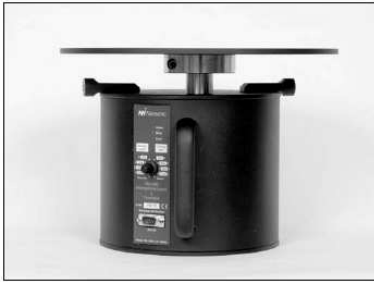
Fig. 1. Norsonic NOR265 turntable. Max load: vertical – 50 kg, Resolution: 0.01^\circ Rotation speed: from 22.7 to 720 s/rev. Turntable plate dimensions: 300 mm Weight: 6 kg Drive: stepper motor.
