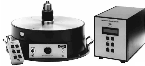
Fig. 2. Brüel&Kjær type 9640 turntable. Max load: vertical – 100 kg, horizontal – 30 kg Resolution: 1^\circ Rotation speed: from 22.7 to 720 s/rev. Turntable plate dimensions: 354 mm Weight: 12 kg Drive: DC motor.
