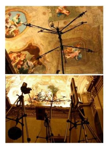
Fig. 1. Typical layout of eight microphones and multiple loudspeakers during the measurement of room impulse response.
