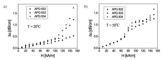
Fig. 3. Changes in the  $\Delta \alpha$  as a function of magnetic field for sweeping time t = 5 min and the temperature: a)  $T = 20^{\circ}$ C and b)  $T = 50^{\circ}$ C.
