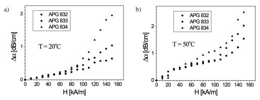
Fig. 2. Changes in the  $\Delta \alpha$  as a function of magnetic field for sweeping time t = 10 min and the temperature: a)  $T = 20^{\circ}$ C and b)  $T = 50^{\circ}$ C.
